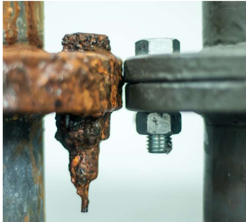
ASTM B117, 10,000 hours in a Hot Salt Fog Chamber (Left, control sample) - (Right, Enviropeel protected sample)
